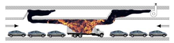
Fig. 2. An exhaust ventilation system with large extraction vents that can be opened close to the site of a fire will protect cars and passengers from smoke and fire gases, and will allow the fire brigade to attack the fire from two sides.
